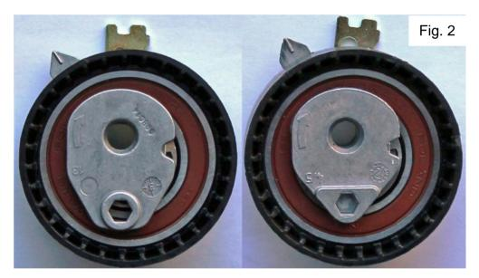
The old belt (5501XS), old tensioners (T43064 and T43168) and kits from your inventory can still be installed on K4J/K4M applications manufactured before 2013. Old generation parts and new generation parts can't be mixed. The new belt (5671XS) may be used on all K4M/K4J applications. However, it must only be used in conjunction with the new generation tensioners (T43236 and T43238).
