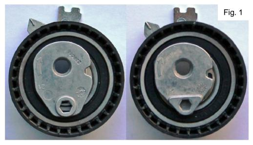
An OEM/OES upgrade has made timing belt 5501XS and the associated tensioners T43064 (Fig. 1 left) or T43168 (Fig. 1 right) as well as the related kits, obsolete. They will no longer be installed on Renault K4M/K4J engines.
